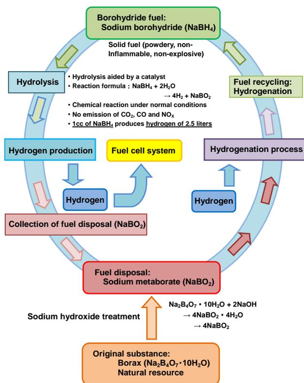
**Fig.1 Hydrogen generation from SBH and recycling of used SBH**
