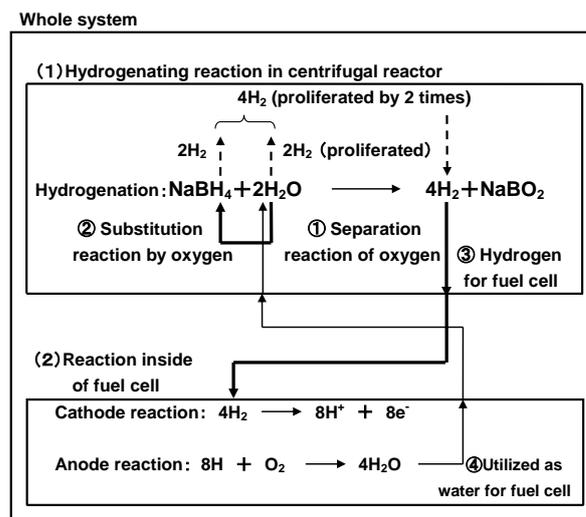
**Fig. 4 Flow of proliferated hydrogen and water**
