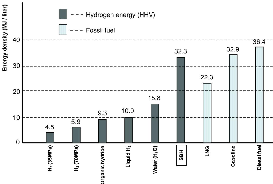
Fig. 6 Energy density of various fuels which consist of hydrogen compound
