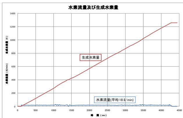
**Fig. 3 Flow rate and cumulated volume of H<sub>2</sub> generated by the centrifugal reactor**
